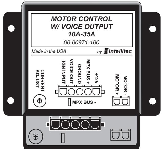
motors are at rest. As the switch is depressed (In or Out direction) each function sends a different load to the module which in turn interprets the direction of travel.
