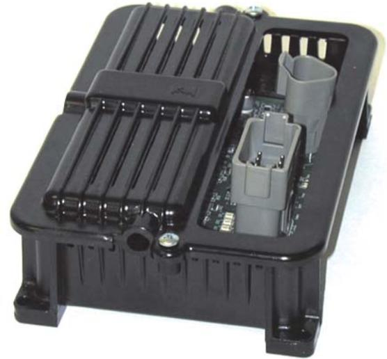
The approximate module dimensions are 7.25" X 4.75" X 2.25" (184mm X 121mm X 57mm).
